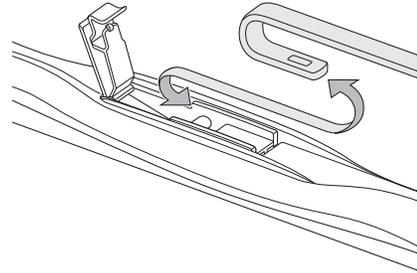
3. Lock wiper arm in place by pressing down on the securing clip.
